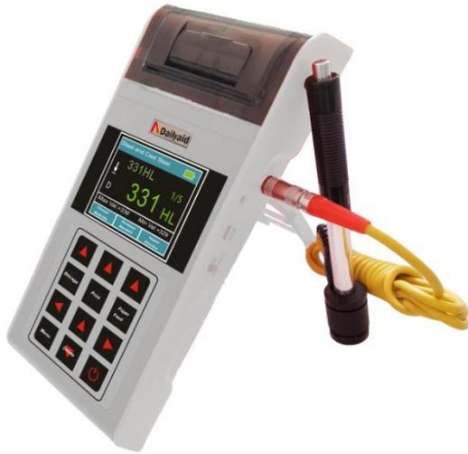
◎An integrated portable Leeb hardness tester with printer, which is convenient for the user to print the testing results, particularly suitable for the outgoing hardness testing, is the most cost-effective portable hardness tester.
